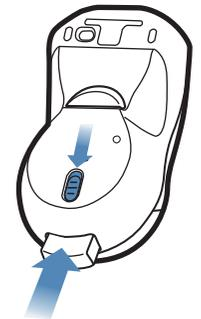
14 Insert the USB Receiver into the USB storage compartment. Push gently until it clicks in place. Push gently again to release.
