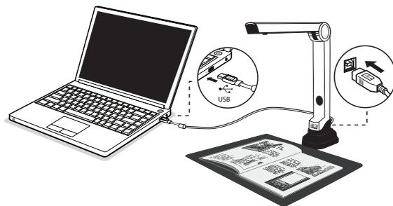
2. Adesso Cybertrack 510 will connect automatically to your computer. (Adesso Cybertrack 510 is a driverless device used with Windows 10, 8, 7, Vista or XP operating systems. Your computer will recognize the device under the Cameras in the Windows Device Manager menu.)
